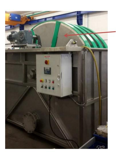
Filtration elements in stainless steel from 10 to 100 microns spacing
