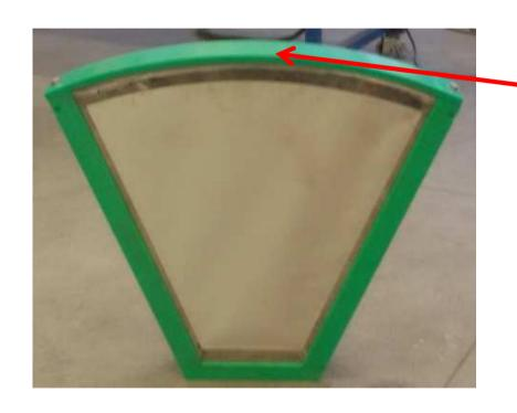
Each filtration element can be inspected and eventually replaced very easily. It is only necessary to remove the top cover. After removing the top cover it is possible to extract the element to check it or to replace it with a new one
