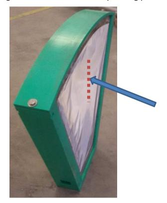
The major resistance of the stainless steel filtration element gives the possibility to wash the filter more frequently. This possibility will increase the efficiency of the disk filter
