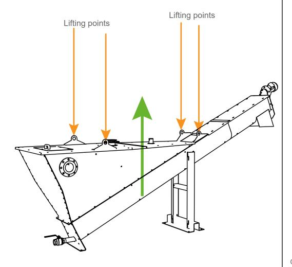
Lift up CDS unit connecting crane hooks to the 4 lifting points
