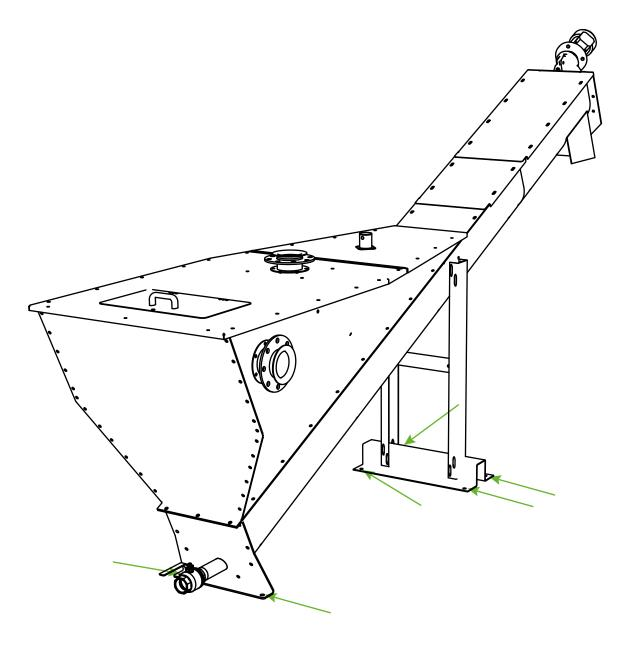
Place back the CDS matching each thread bar and following the scheme here on the right bolt them all.
