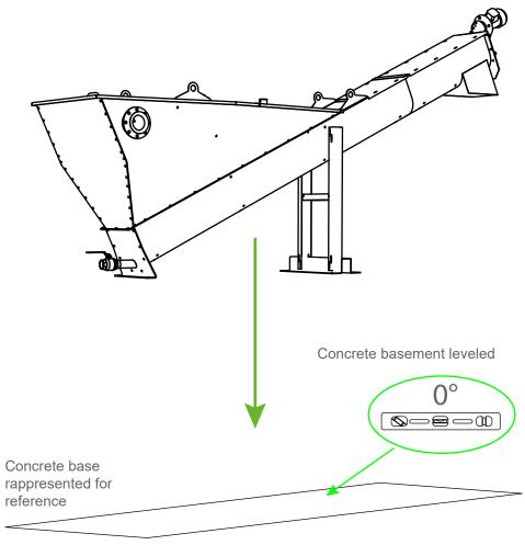
Locate the CDS on the concrete basment
