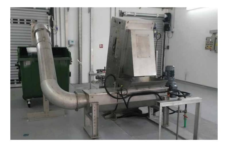
The CPP - SCREW SCREEN PRESS simultaneously provides the function of drainage and waste compaction. The compactor can be placed directly below the output of a coarse filtration machine or it can be fed by a conveyor.
